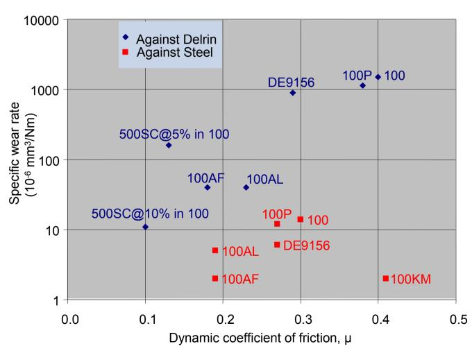
For metal as a counter surface, the harder the surface the better the wear and friction behaviour of the system. Aim for a hardness of greater than 50 HRC
